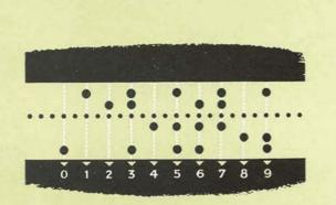
Data are represented by holes punched in paper tape. The digits 0 to 9 are all represented by rows containing an odd number of holes. This allows them to be checked, for should an error have occurred and one hole be dropped or an extra one put in, the resulting character would not be a number but some other symbol. On input the check is made by the computer; on output any such error would be immediately apparent.
