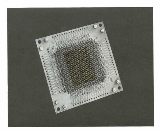
An outstanding feature of the Ferranti Mercury Computer is that magnetic cores are used for the store in which all computation is carried out. These cores are mounted in square arrays of 32 by 32. The typical plate illustrated above contains two such arrays, one on either side. The central coloured area in the photograph has been enlarged and used as a background on the front cover of this brochure.
