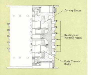
The backing store consists of four magnetic drums, each rotating at 3472 r.p.m., and having a storage capacity of 4096 40-digit words. Every group of 10 digits in the backing store has a check digit associated with it; this digit is referred to whenever a transfer is made to the computing store. Any error in operation will be detected and the machine will indicate this and stop.
